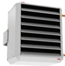
Fan heater SW is designed for heating of industrial premises, work shops, storage rooms, supermarkets, etc. Modern fan technology optimises the air flow through the heater battery, achieving sound levels as low as 35 dB(A). The balanced motor and axial fan combination supplies a smooth flow of heat from the water coil. Provided with air directors. The fan heater can be wall or ceiling mounted with water connection on either side. Regulation of air flow in three stages
